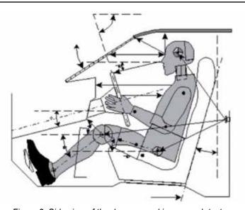
*Figure 2. Side view of the dummy used in car crash tests* Source: Report number: NCAP-CAL-15-003, New Car Assessment Program (NCAP), Frontal barrier impact test, Toyota Motor Corporation, 2015 Toyota RAV-4 SUV, pp. 14 (2–8).
